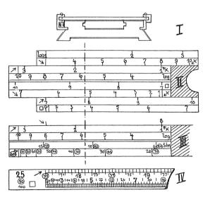
Fig I is a cross-section, Fig II is a schematic of the whole front of the rule, Fig III is a schematic of the back of the slide,
